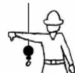
**LOWER BOOM** – With arm extended horizontally to the side, thumb points down with other fingers closed.
