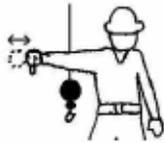
**LOWER THE BOOM AND RAISE THE LOAD** – With arm extended horizontally to the side and thumb pointing down, fingers open and close while load movement is desired.
